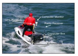
Figure 7. Oregon State University's Coastal Profiling System set-up, which allows access to shallow sections of the estuary. Source: Wood and Ruggiero 2014
