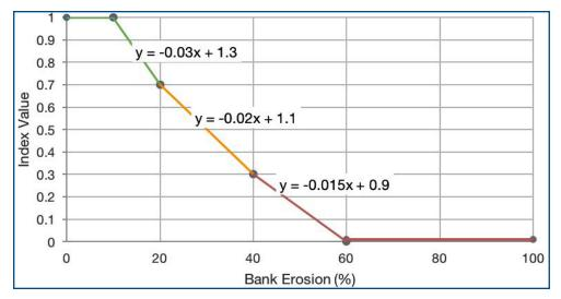
Figure 4.18 Bank Erosion Standard Performance Index
